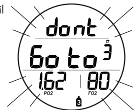
Fig. 120 - GAS SWITCH WARNING
